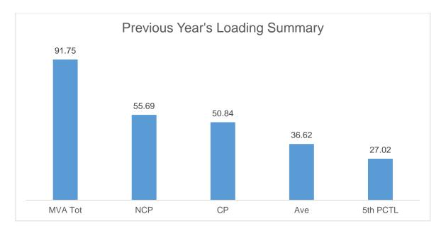
The Non-Coincident Peak Demand is 55.69 MW, which is around 60.70% of the total substation capacity of 91.75 MVA at a power factor of 0.85. The load factor or the ratio between the Average Load of 36.62 MW and the Non-Coincident Peak Demand is 65.76%. A safe estimate of the true minimum load is the fifth percentile load of 27.02 MW which is 48.52% of the Non-Coincident Peak Demand.
