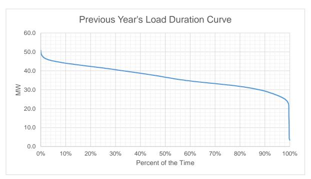
Based on the Load Duration Curve, the minimum load is 3.36 MW and the maximum load is 50.84 MW for the historical year.
